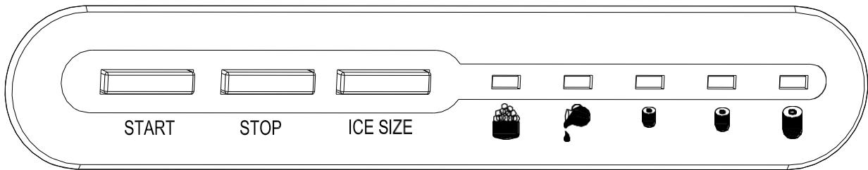
**'START'** and **'STOP'** button: When the power is connected, the unit will enter the standby status(the ice selection mode light will flash); when pressing the '**START**' button, (the related ice selection light will turn green), then the unit starts to work. When press the '**STOP**' button, the unit will be back to the status of standby;
