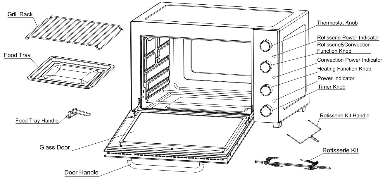
**Temperature Knob:** choose the desired temperature from 90°C to 230°C.
